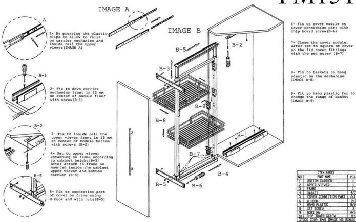
7- Close the cover module. After set to square ot cover on the lid cover fittings with the set screw (B-7)
